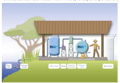
electrically operated pump. In the first step organic and anorganic solids are to be separated. The water is then passed at low pressure through special ultrafiltration membrane that holds back contaminants that are invisible to the naked eye: pathogenic and coliform bacteria filtered out completely, and 99.9999% of viruses removed. This corresponds to a "logarithmic removal value"
